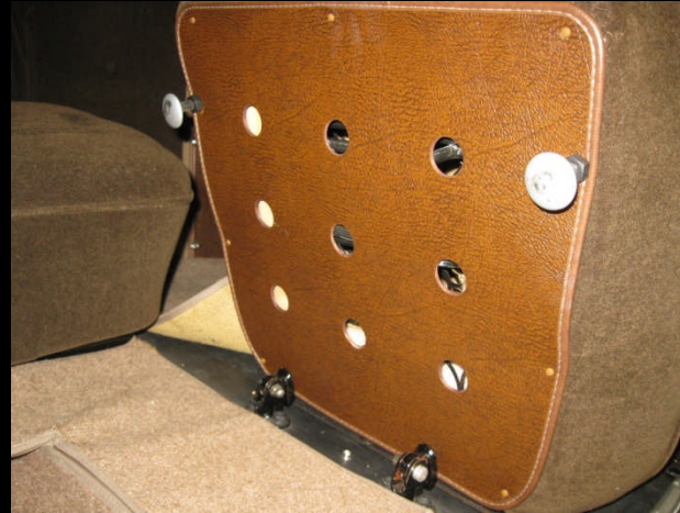
190-A Late Passenger Seat folds and tips forward for easy entry into the back. The seat bottom is brown dash grain cardboard, the rests are cad plated.
