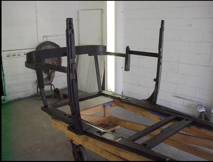
A-400 wood sub-frame door pillar and the rear belt rail.
