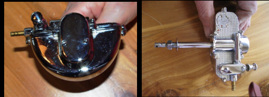
Trico vacuum windshield wiper motor TR-C2B
