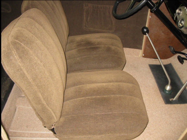
Victoria front seats have 5 pleats & were covered in Brown Mohair, Brown Bedford Cord or Tan Broadcloth.
