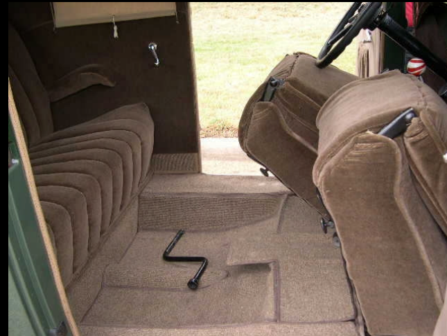
190-A Early Seats The driver & passenger seats fold for entry into the back. The seats are attached to "L" brackets on the floor. The drivers seat is adjustable with three holes in the bracket, while the passenger seat is fixed.
