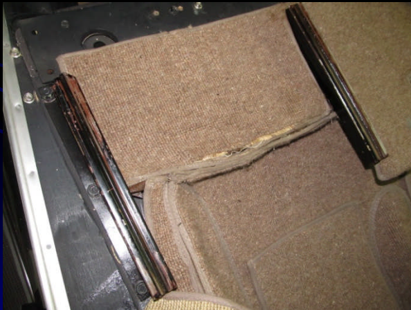
190-A Late Style Driver seat tracks similar to those of 400-A, introduced in mid June 1931
